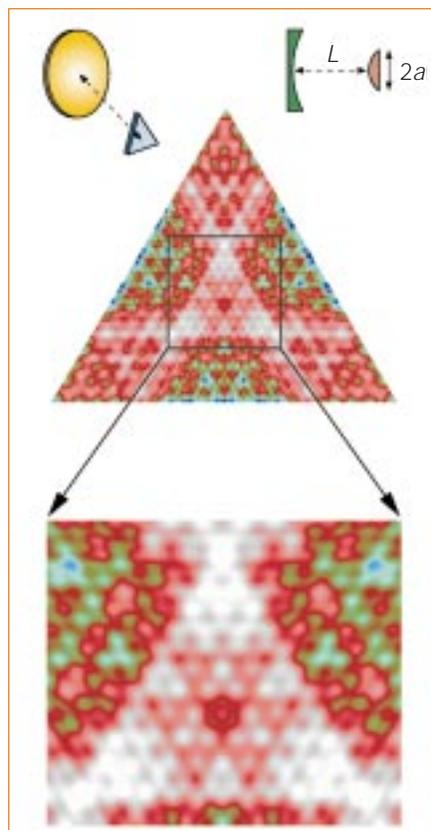
**Figure 1** Calculated lowest-loss eigenmode of an unstable resonator with a triangular mirror. Left inset, a three-dimensional view; right inset, a side view.  $M = 1.5$ ,  $N = 10.5$ . The intensity distribution  $|u|^2$  on the small mirror is shown: white, high; red, medium; blue, low. Bottom, magnification of the centre part, with colour coding adjusted to exploit the full dynamical range.
