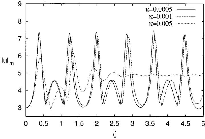
Figure 2. Peak amplitude of  $N=3$  soliton beams showing the modification of the soliton period and then the breakdown of periodicity as  $\kappa$  varies from 0.0005 to 0.005.
