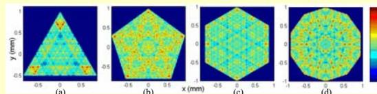
FIG. 5. Detailed two-dimensional fractal modes of unstable resonators with (a) triangular, (b) pentagonal, (c) hexagonal, and (d) decagonal output mirrors. The cavities have a magnification of  $M = 1.5$ , and an equivalent Fresnel number, defined in [1-4], of  $F_{\text{eq}} = 50$ .
