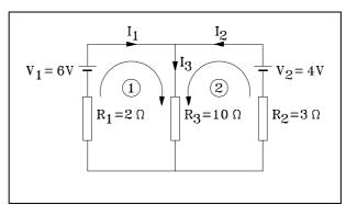
From the node rule:  $I_1 + I_2 - I_3 = 0$  1. From the loop rule:
