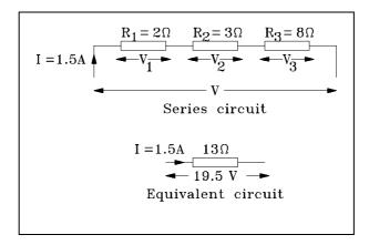
In this series circuit the voltage drop across each resistor is:
