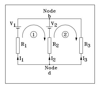
If we use Kirchoff's law to analyse the current through the circuit, then the first step is to assign a sense to the current in each of the branches of the circuit - this can be done completely arbitrarily as if you get it wrong then the value of the current will be negative. In this circuit the chosen direction of the 3 currents  $I_1$ ,  $I_2$  and  $I_3$  is upwards. There are 2 nodes at b and d and so if we apply the node rule we obtain:
