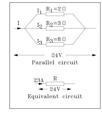
$I_1 = V/R_1 = 24/2 = 12 A$   $I_2 = V/R_2 = 24/3 = 8 A$  $I_3 = V/R_3 = 24/8 = 3 A$
