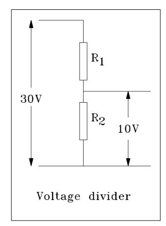
$V_o/V = R_1/(R_1 + R_2)$ 10/30 =  $R_1/(R_1 + R_2)$
