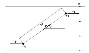
In a uniform electric field **E**, the dipole with moment **p** makes an angle  $\theta$  with the field. Two equal and opposite forces **F** and -**F** act on the charges (couple) and are equal to:
