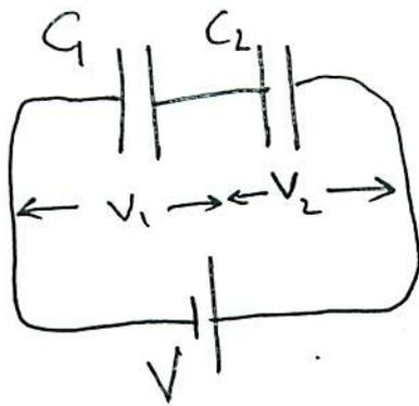
● One may envisage a gravitational potential analogy to see that the individual potentials ( $V_1$  and  $V_2$ ) add up to the potential  $V$ . ... it is like climbing a ladder in two stages
