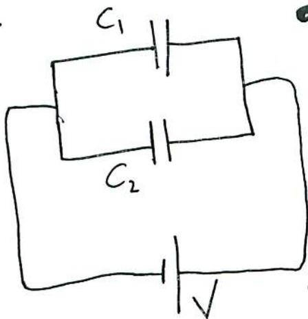
• In parallel, the potential difference  $V$  is across both capacitors, i.e.  $V$  is the same for both.
