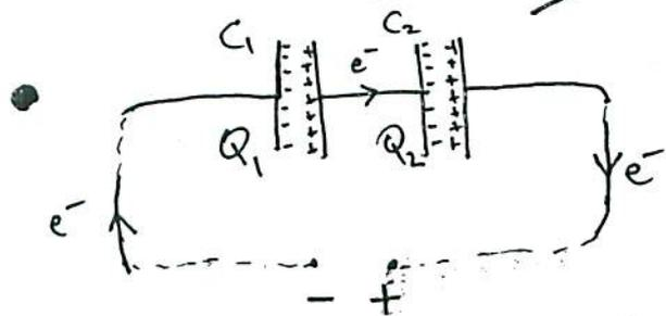
Electrons build up on the left plate of  $C_1$ . These repel electrons in the connecting wire towards  $C_2$ . Electrons are then repelled from the right plate of  $C_2$  towards the battery.
