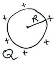
Outside, and on the surface, the potential is the same as if the charge  $Q$  is all at the point at the centre of the sphere. (5)
