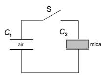
Consider two parallel plate capacitors of identical dimensions, one of which has air as the dielectric and the other mica. The air capacitor is charged to 400 V, isolated and then connected (via a switch S) across the mica capacitor, which is initially uncharged (see the above diagram). Once the switch is closed, the potential difference across this parallel combination of capacitors becomes 50 V.
