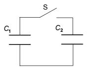
A capacitor of capacitance  $C_1 = 10 \ \mu\text{F}$  is charged so that the potential difference between its terminals is  $V_1 = 50 \text{ V}$ . The terminals of an uncharged capacitor, with capacitance  $C_2 = 2.5 \ \mu\text{F}$ , are then connected to those of the charged capacitor (see the above diagram).
