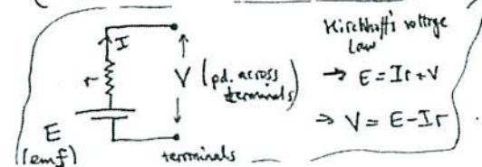
$$\begin{aligned} V_1 &= E_1 - I_1 r_1 = 12 - (0.6)6 = 8.4 \text{ V.} \\ V_2 &= E_2 - I_2 r_2 = 8 - (-0.08)4 \\ &= 8 + 0.08 \cdot 4 \\ &= 8.32 \text{ V.} \end{aligned}$$
