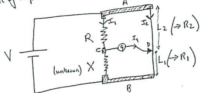
Balance condition arises when  $I_g = 0$  (as a result of the same potential at points C and D)
