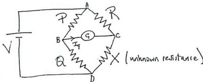
'At balance':  $I_g = 0$  i.e. points B and C have the same potential
