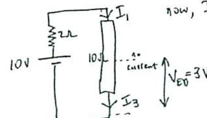
$$\text{now, } I_1 = I_3 = I, \text{ say} \quad I = \frac{10 \text{ V}}{(2+10) \Omega} \text{ (ohm's law)}$$
