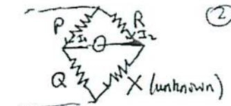
$$\left. \begin{array}{l} P = 1000\Omega \\ Q = 0.5\Omega \\ R = 1000\Omega \end{array} \right\} \rightarrow X = \frac{0.5 \times 1000}{1000} = 0.5\Omega.$$
