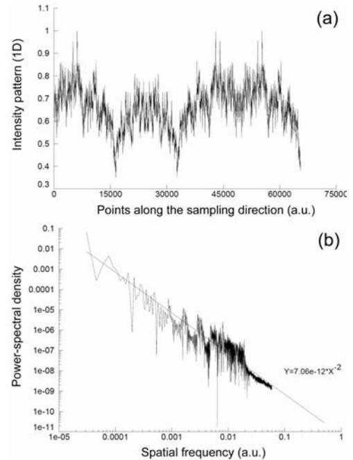
Fig. 4. (a) Slice through the lowest-loss mode of a triangular kaleidoscope laser with  $N_{\text{eq}} = 703.3$  and  $M = 1.9$  (sampling line passing through a vertex and perpendicularly through the opposite edge). (b) BENOIT power spectrum calculation and best-fit line [whose slope is directly related to the fractal dimension of the pattern shown in part (a)].
