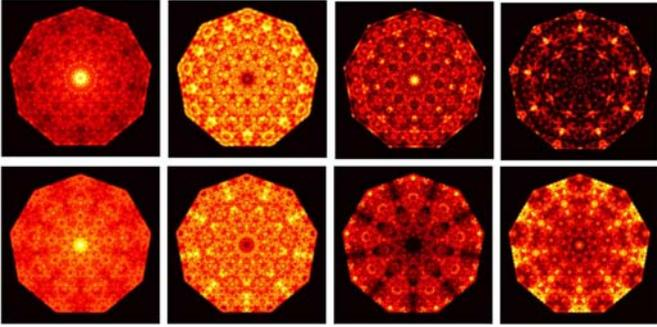
Fig. 2. Lowest-loss mode and first three higher-order modes (left to right) for a kaleidoscope laser with  $N = 9$  and  $M = 1.5$ . Top row:  $N_{\text{eq}} = 20$ . Bottom row:  $N_{\text{eq}} = 30$ .
