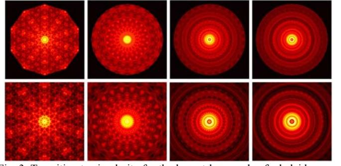
Fig. 3. Transition to circularity for the lowest-loss mode of a kaleidoscope laser with  $N_{\text{eq}} = 30$  and  $M = 1.5$ . The lower panes show a magnification of the central portion of the pattern. The number of aperture edges in each case is (left to right):  $N = 10, 20, 30,$  and  $40$ .
