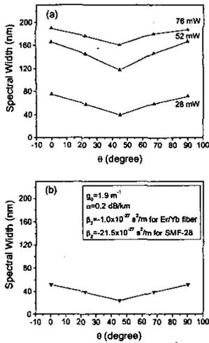
**QThE5** Fig. 3. The polarization angle dependent spectral width of the CRSS is shown for the results of (a) three different optical pump powers and (b) the simulation results for 17 mW. The inset is the parameters used for the simulation.
