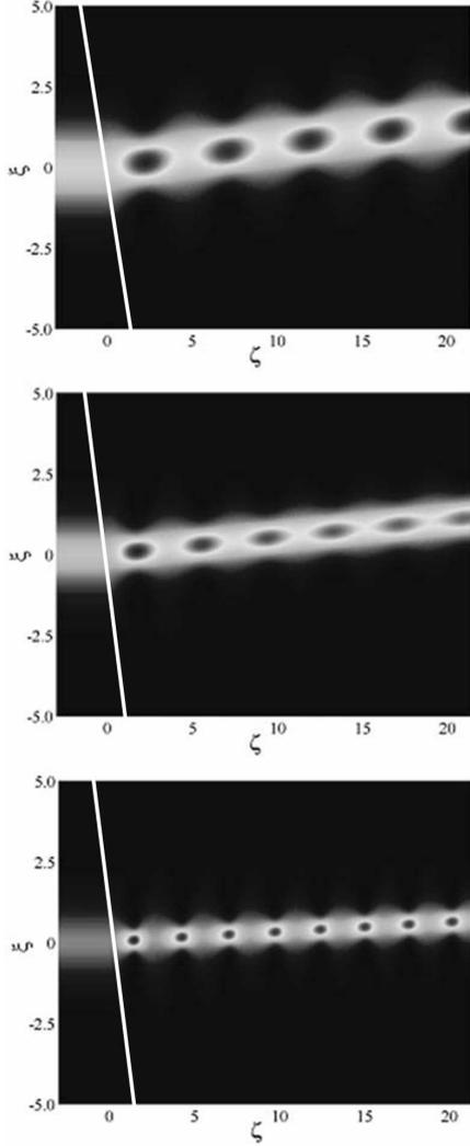
Figure 2: Refraction of spatial solitons at a nonlinear interface between power-law type media with similar nonlinearity exponents (the refractive index varies as  $\delta n_{\text{NL}}^2 \sim I^p$ ). The incidence angle in each part is  $30^\circ$  (well beyond what is attainable from paraxial theory [1-6]). Top:  $p = 1/2$ ; middle:  $p = 1$  (Kerr); bottom:  $p = 3/2$ .
