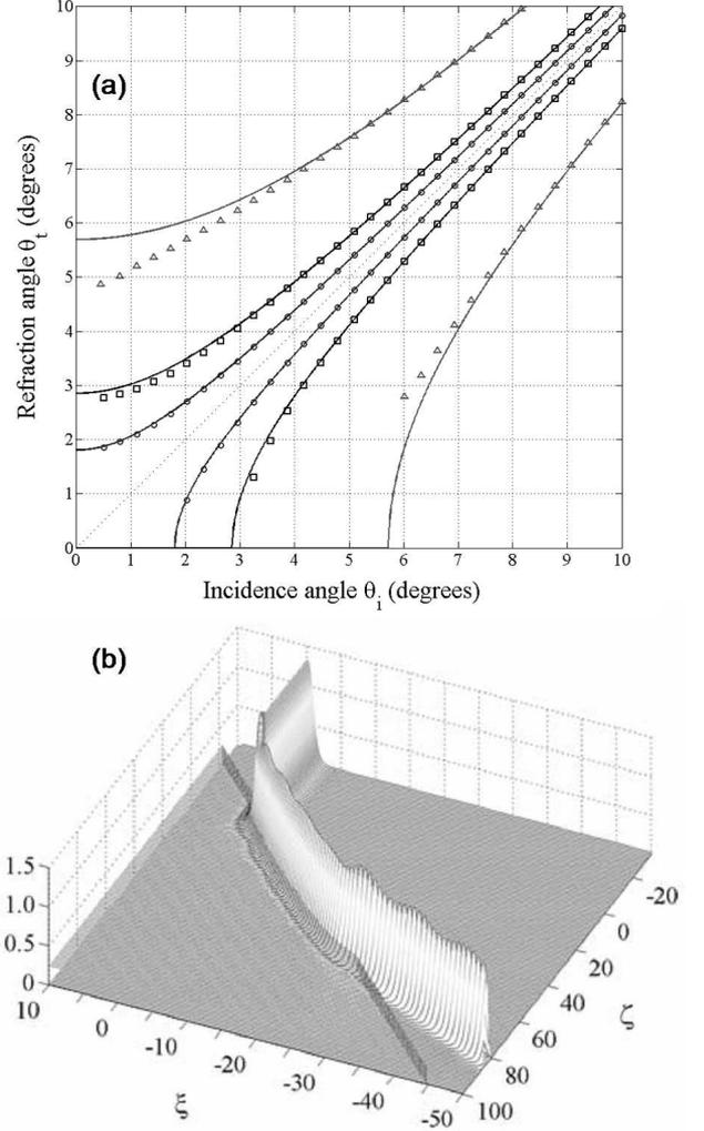
Figure 3: (a) Extensive computations have tested the validity of Snell's law (3), here for Kerr/cubic-quintic interface scenarios. (b) Goos-Hänchen shifts can occur when incidence angles are close to the critical angle.
